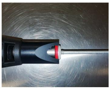
**Fig. 2** Example of a depth-locating nose piece with tapered sides
